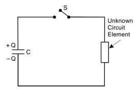
In the circuit above, the capacitor is initially charged. If the switch is closed, an alternating current will be produced if the unknown circuit element is:
