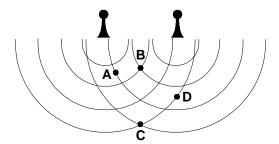
The diagram represents the wave fronts of two sound waves. The waves are in phase and have the same frequency. At which point on the diagram is the sound loudest?
