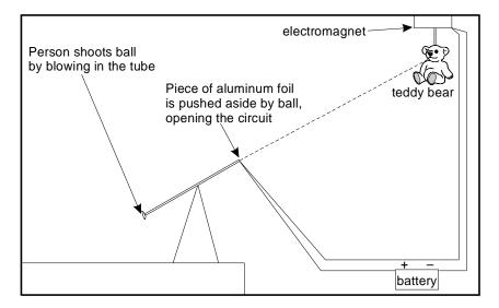
The diagram shows a blowgun aimed to shoot a small ball at a teddy bear. The teddy bear is suspended by an electromagnet. When the ball leaves the blowgun, the electromagnetic circuit is opened and the teddy bear is released. This apparatus is most useful for demonstrating:
