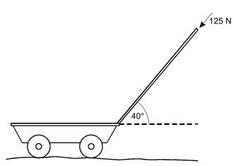
A garden cart of mass 22 kg is pushed on level ground with a handle that makes an angle of  $40^{\circ}$  with the horizontal. A force of 125 N is applied along the direction of the handle as shown.
